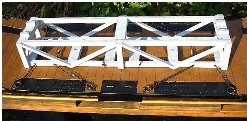
The final result is shown below. Note the Boilers are chained to the Cradle.
