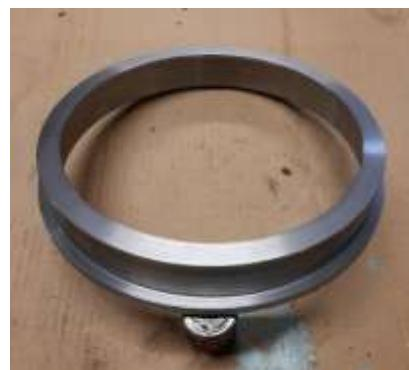
very close fit for the Loctite is nearly as bad as pressing it on as the Loctite starts to go off as soon as it is enclosed, but at least heating it softens the Loctite for another go.
