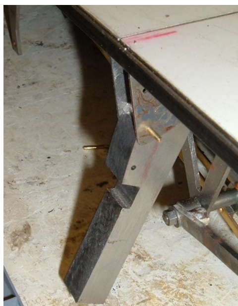
Dropped Post, showing Support Trunnion
