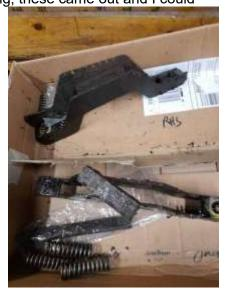
As an aside, it is interesting to see these bits and pieces as they have 'loco history' imprinted on them, with the addition of weld, broken and missing screws presumably arrived at 'in situ' to avoid stripping the loco to cure a fault. It is a bit like the use of a taper pin to hold a recalcitrant wheel in place, which was probably also applied without stripping the loco. In fact, I have a very vague
