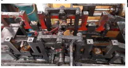
cylinders, crossheads, guides and valve gear in place and, where required, paint around the fixings. None of the pivots in the valve gear or crossheads look excessively worn, although I have been contemplating making a crosshead water pump for it if I can work out mounting and drive. I am not overly keen on water for a
