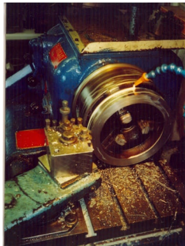
Preparing the tread on a flame cut ring. The original surface can be seen on the inside of the ring
