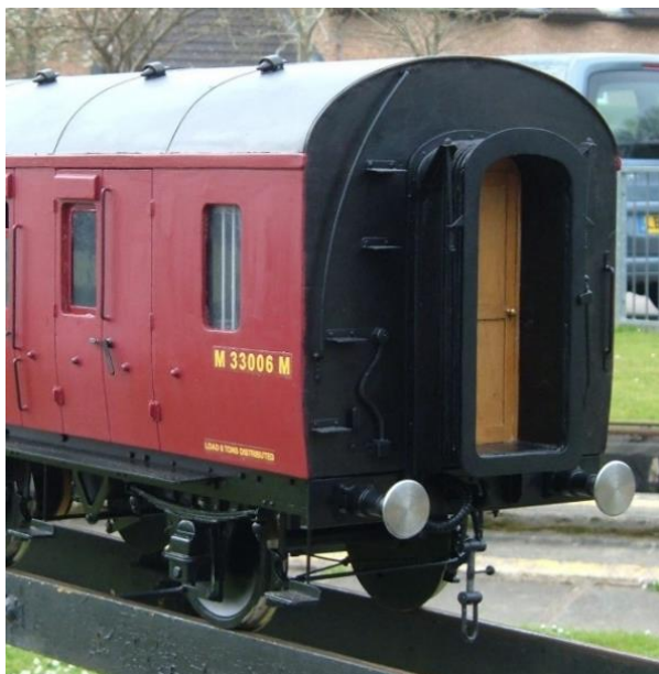
Body Profile and End Steps, Handrail and Gangway.
