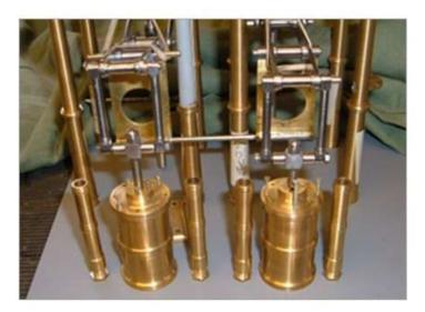
Eccentric straps were roughed out in the mill and parted-off, to be finished by hand filing. I tackled the eight tapered brass columns supporting the steel entablature by making each in three parts, screwed together.
