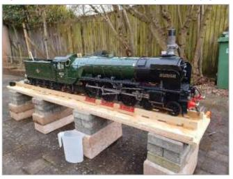
reasonably well with the loco actually running smoothly. It did however throw up a problem with a cylinder cover gasket leaking which needed some urgent attention. The gaskets I made from sheet material and now fit them with light smear of Hermatite Red compound. Final checks were OK and ready for the Steam Test.
