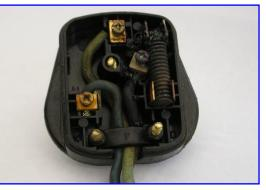
was taken out, this often happens with old TRC (tough rubber covered) cable, and was reconnected within the equipment. I felt that I should check the wiring within the plug and removing the cover showed the heat damage caused by obvious overloading. Fortunately, there was a 30amp supply in the workshop, and after fitting the appropriate plug the equipment was checked and found to be in working order. The actual current drawn by the unit was 22.5 amps.
