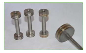
The final task for this update, which is as I write on the workshop bench, is the inner connecting rod. Another simple looking job that consumes more hours than you first expect, but on the home run now, just need to make and fit the clamping studs and then bore the hole for the main bearing. Of course, then the whole thing needs the obligatory tidy up with emery paper etc.
