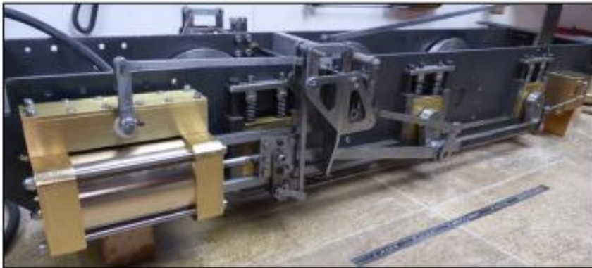
Two views of the actual loco chassis during testing
