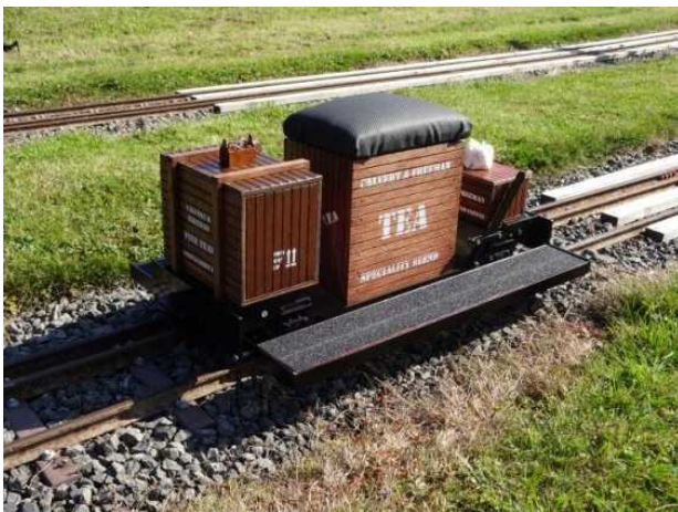
Photo 2: Ground/raised-level riding truck in 5" gauge
