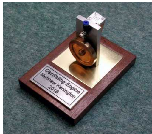
Photo 2: Matthew's oscillating engine (from bar stock) – serialised in EIM
