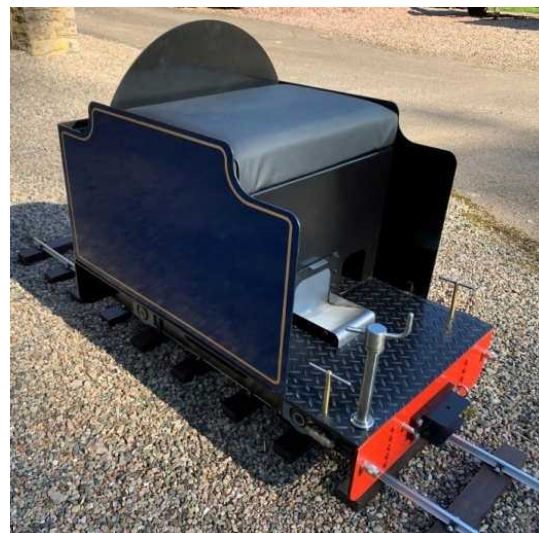
Photo 3: 7 1/4" gauge riding truck/tender (designed from scratch in 3D CAD and serialised in EIM)
