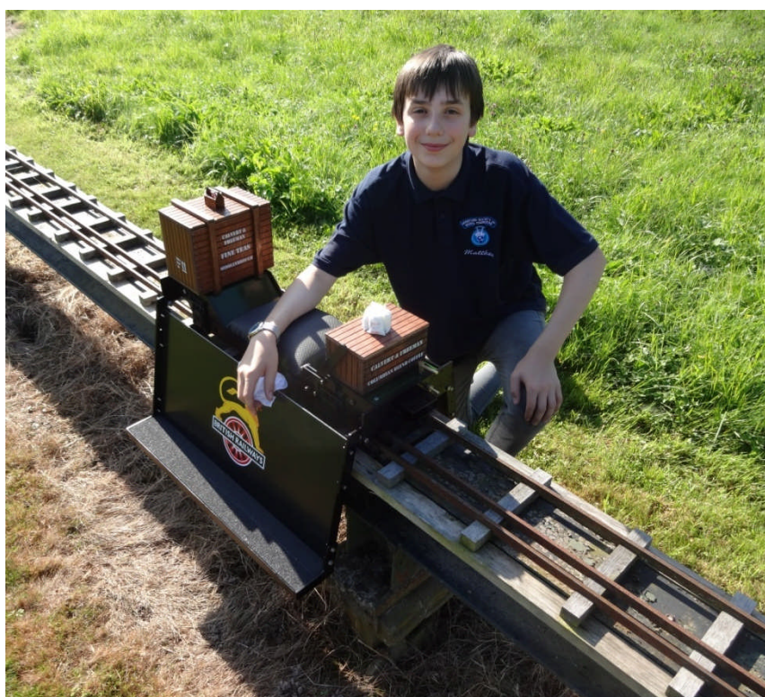
Photo 1: My son, Matthew, with one of the projects he built at Hereford SME's Young Engineers Club – a combined ground and raised-level riding truck/tender for 5" gauge
