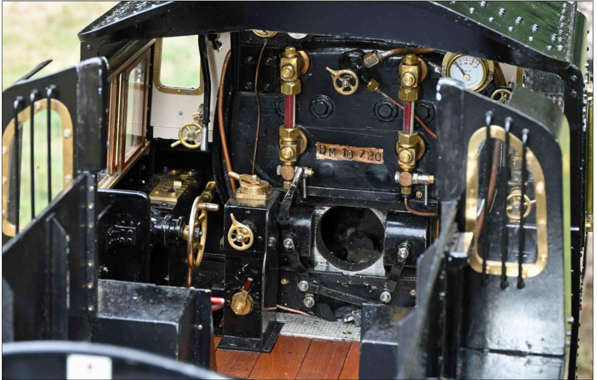
Blower valve and control for steam drain cocks mounted on pedestal to right of reverser which also carries a dummy vacuum brake lever.
