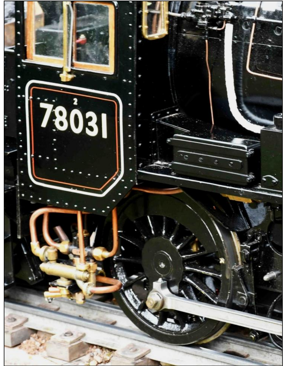
AWS battery box.
