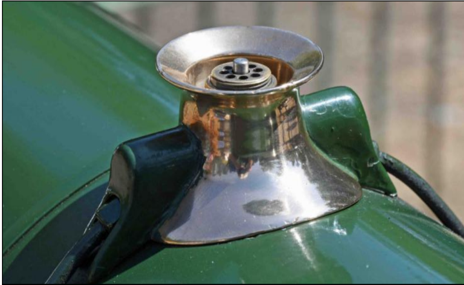
Martin's own efficient design pop valve in GWR housing.
