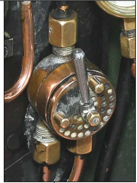
Steam brake valve made to look like a vacuum brake valve.
