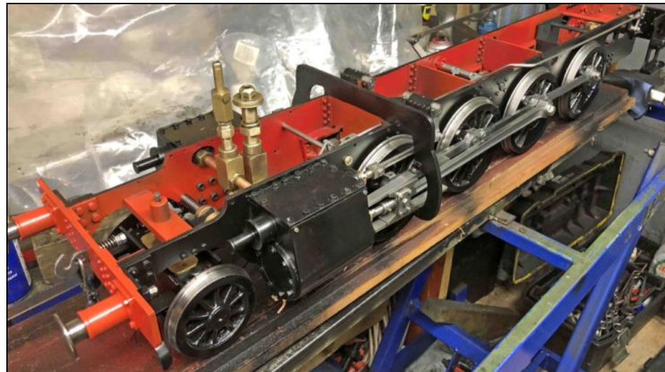
Completed chassis ready for air testing.
