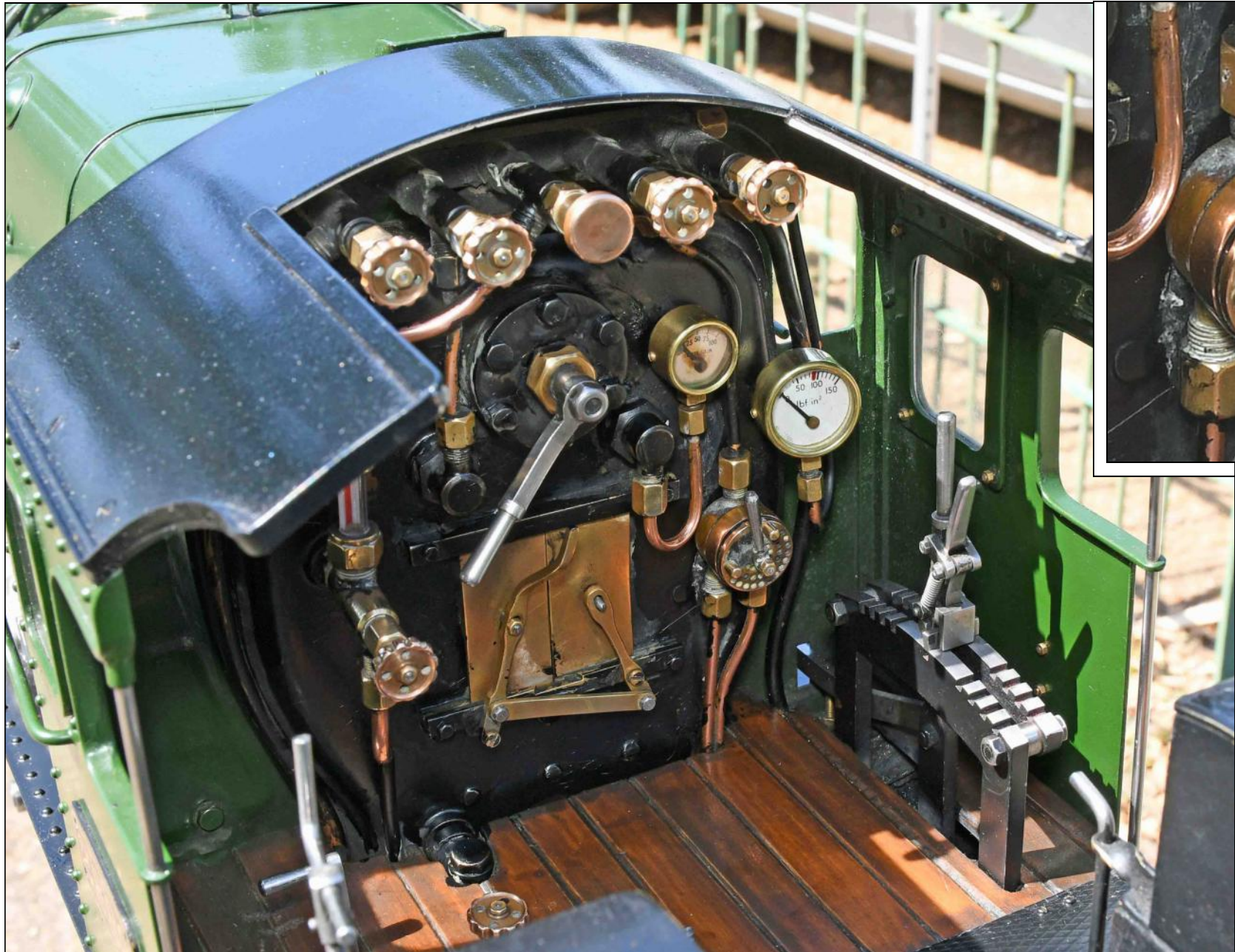
Steam brake valve made to look like a vacuum brake valve.
