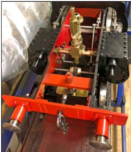
Slide valve cylinders with temporary connection for air testing.
