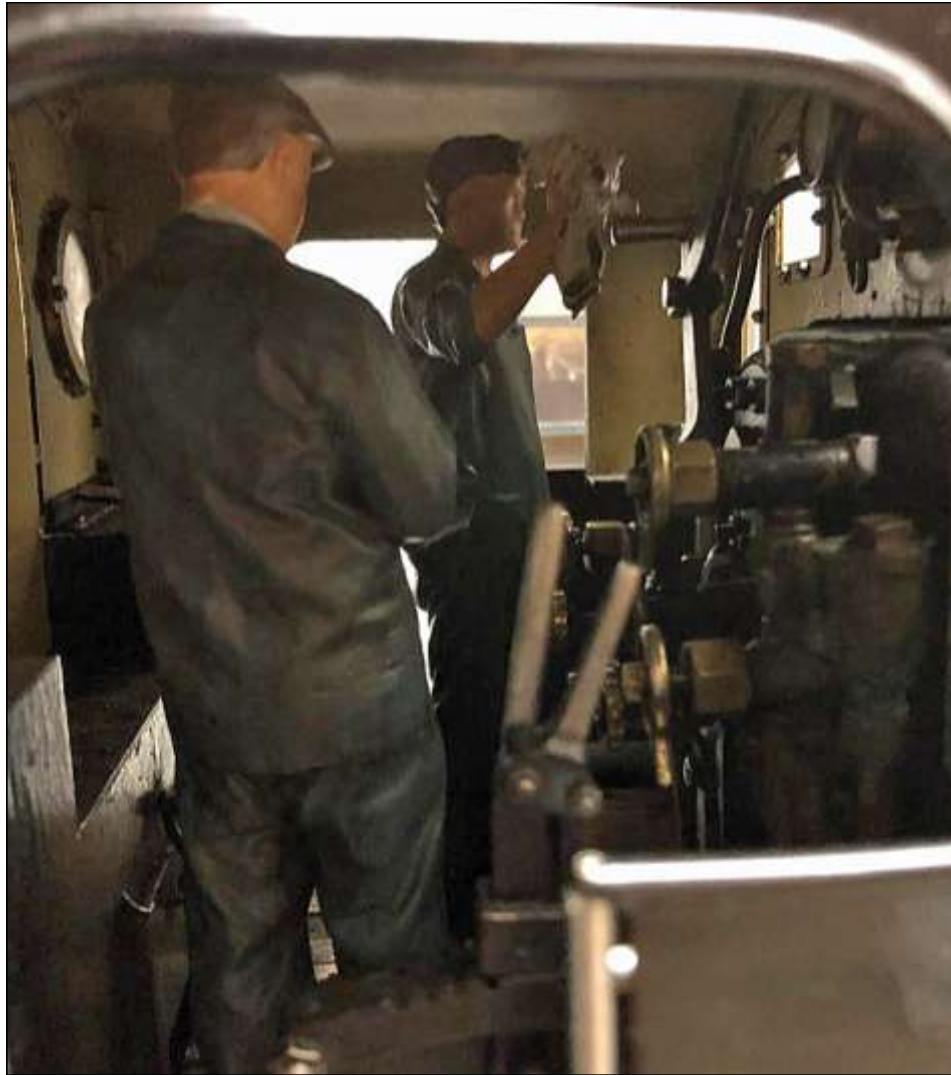
Designed and built by Andrew Hardy as a small scenic diorama, this interior model of a generic locomotive running shed has been built using CNC machines and 3D printing with every part created from either laser scans or 3D CAD drawings.
