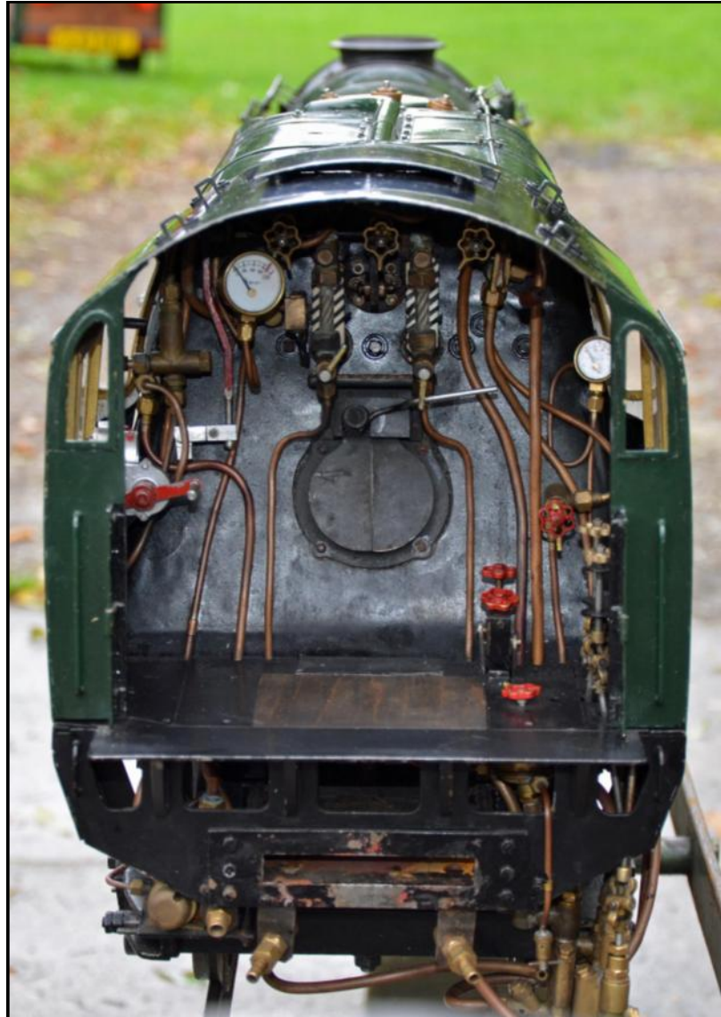
Fitted with four radiant superheaters, the boiler was built using Bernie's own formers, silver brazed using oxy/propane equipment and passed inspection and its 200psi shell test without a problem. Controls on the left of the cab include reverser, vacuum brake (top left) and pressure gauge. Controls on the right of the cab include injector, turbine and damper.
