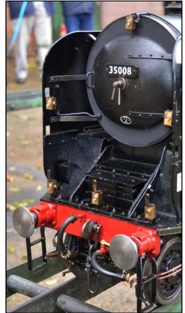
Working headlamps and cab lighting are powered by a functioning miniature steam turbine. Initial plans had been to fit switches to the lamps but their housings were too small for this to be practicable. Vacuum braking is fitted as on the prototype locomotive and the vacuum pipes visible in these views are functional.
