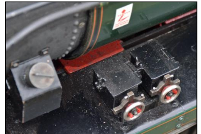
Fabricated vertical injectors (top left) are fitted with innards to DAG Brown's design and work effectively. Working dampers are fitted (top right) and the steam turbine that generates power for headlamps and cab lights is also visible. Dummy sand boxes provide access for axlebox lubrication. Nameplates were designed and etched at home and the lubricators contain working oil pumps.
