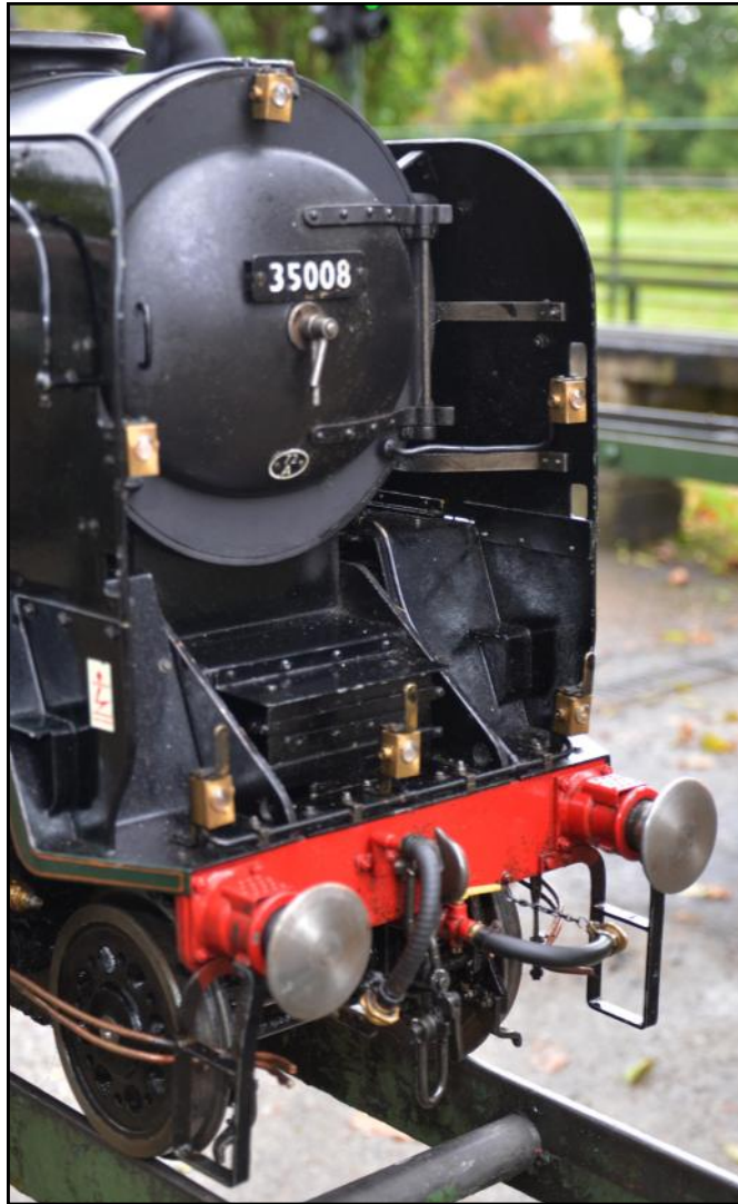
Working headlamps and cab lighting are powered by a functioning miniature steam turbine. Initial plans had been to fit switches to the lamps but their housings were too small for this to be practicable. Vacuum braking is fitted as on the prototype locomotive and the vacuum pipes visible in these views are functional.
