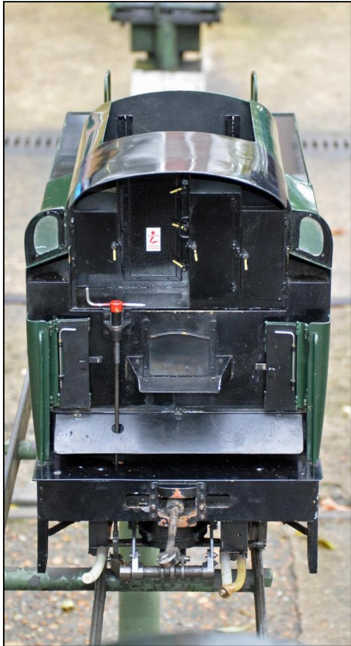
Cupboard doors and doors at the front of the tender (left) all open, the whistle (centre) is a dummy but emits a wisp of steam when blown and the semi-pop safety valves are to Gordon Smith's design. Vacuum cylinders and rear lamps are fitted (right).
