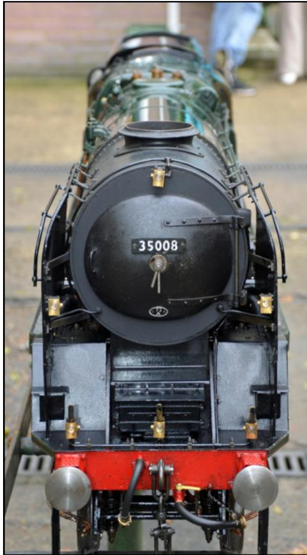
Working headlamps and cab lighting are powered by a functioning miniature steam turbine. Initial plans had been to fit switches to the lamps but their housings were too small for this to be practicable. Vacuum braking is fitted as on the prototype locomotive and the vacuum pipes visible in these views are functional.
