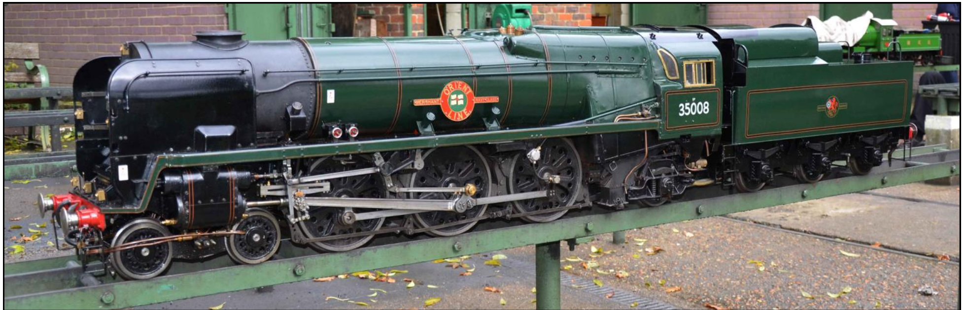
Classic views of Bernard's locomotive at the Maidstone MES Mote Park track reveal a wealth of detail. Construction began in 1990 with wheels cast locally, machined to receive water cut inserts bonded and screwed in place to give the correct Boxpok effect. Balance weights were added and tender, bogie and trailing wheels received similar treatment.
