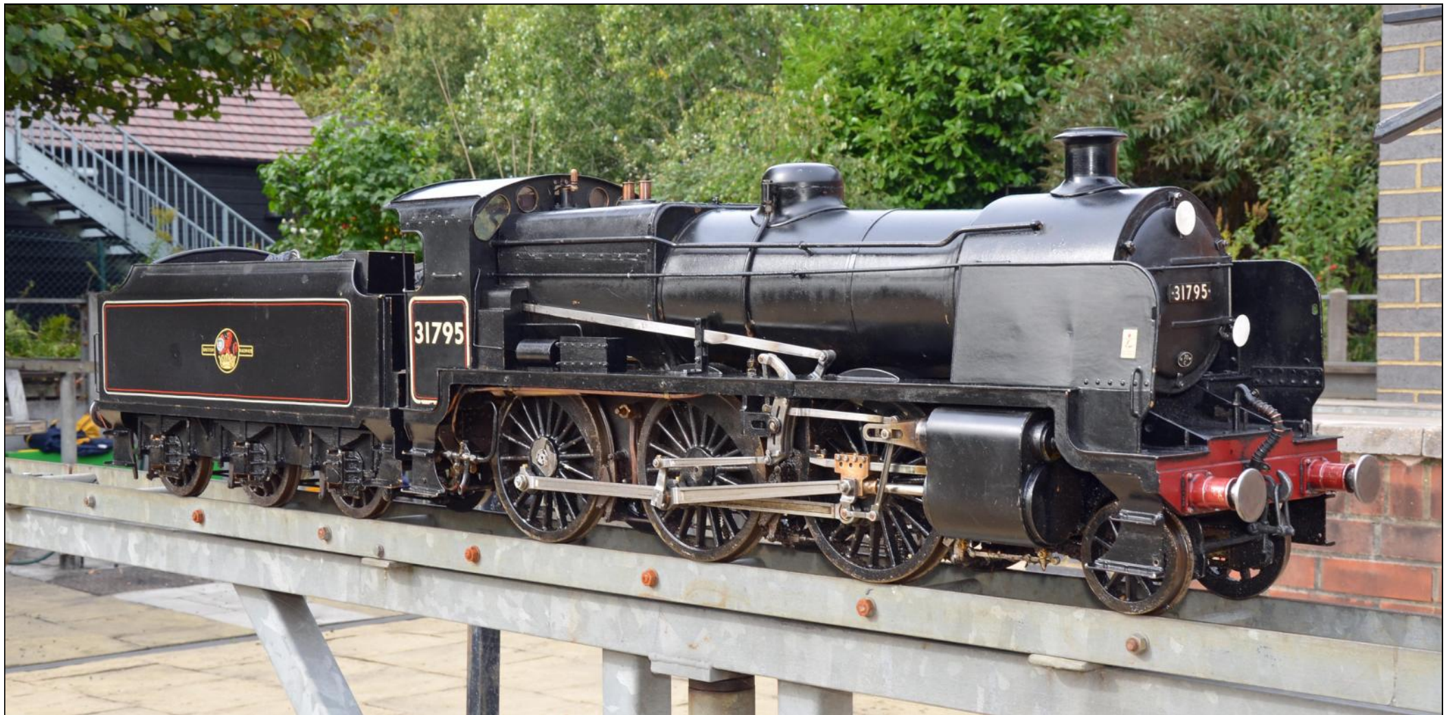
Right hand side three-quarter view. With six London termini and a plethora of possible paths, the Southern used route indicator discs for its trains. Two additional lamp brackets were fitted to the smokebox, giving a total of six rather than the usual four on other regions. There were also six on the tender, for tender first running.
