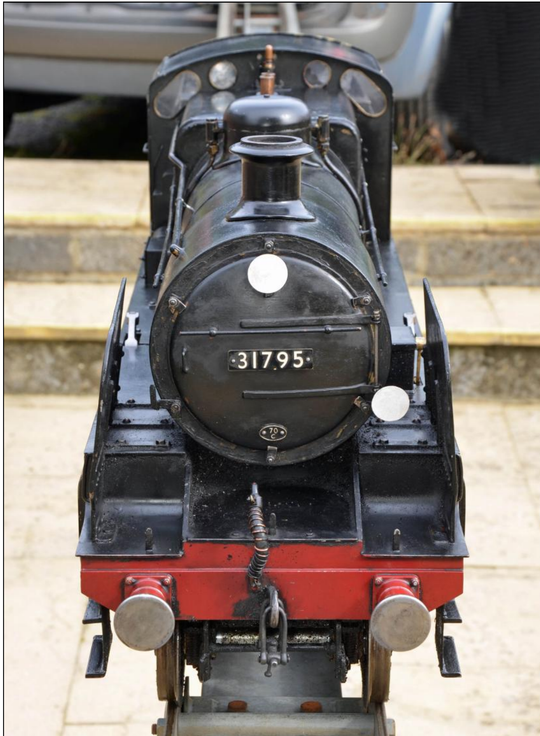
Head on. Note that the smoke box door is locked by six dogs, as per the full-size. It never leaks. The shed plate, fittingly, is for Guildford where several of the class finished their working lives.
