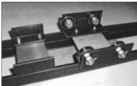
Both rolling roads use the same principle of roller bearings bolted to pieces of angle iron with a spacer plate to suit the gauge. A simple pony truck support is also shown. Each pair of driving wheels sit on a separate roller unit which simply rests on the track. The alternative holes in the angle plates allow the spacing of the roller bearings to be adjusted to suit the wheel diameter.
