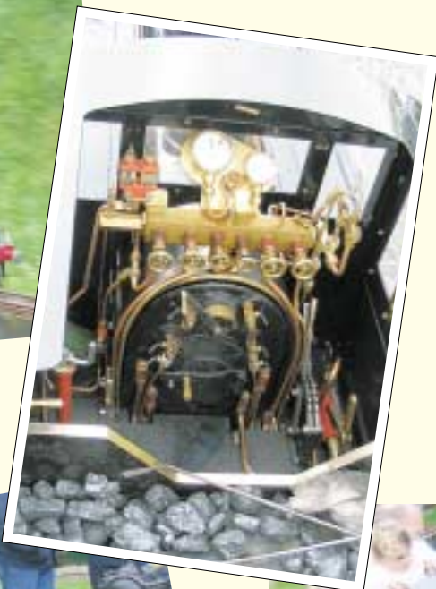
Right: Backhead detail of Denis Mulford's 2-4-2 Baldwin
