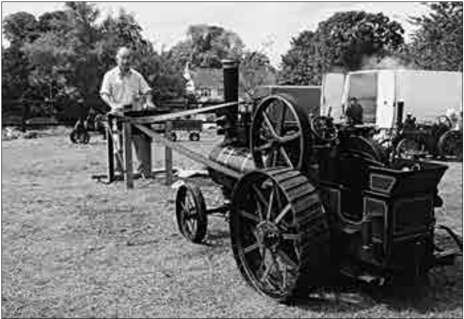
Club member Mike Penny cutting timber, the saw bench being driven by Graham Hunt's 4" scale W & S 8nhp expansion engine Pedler. Graham scaled down from a full size engine, making all his own patterns and castings and built the engine in two years.
