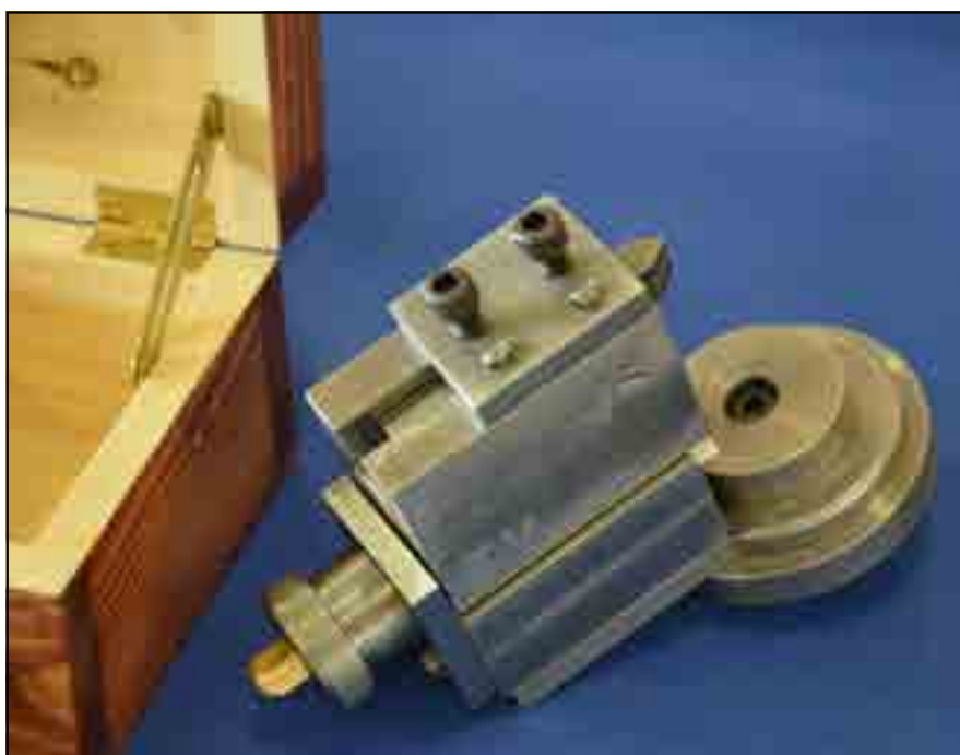
The diversity of model engineering is seen in this 'ball turning' tool exhibited by P Bowler at the recent Doncaster Model Engineering Exhibition. Photo by Mike Crisp
