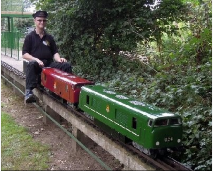
A pair of petrol hydraulic locos running in tandem, the creation of Aubyn Mee, Rugby's Chairman. The power is Honda industrial engines adapted for this interesting role. Photo John Billard
