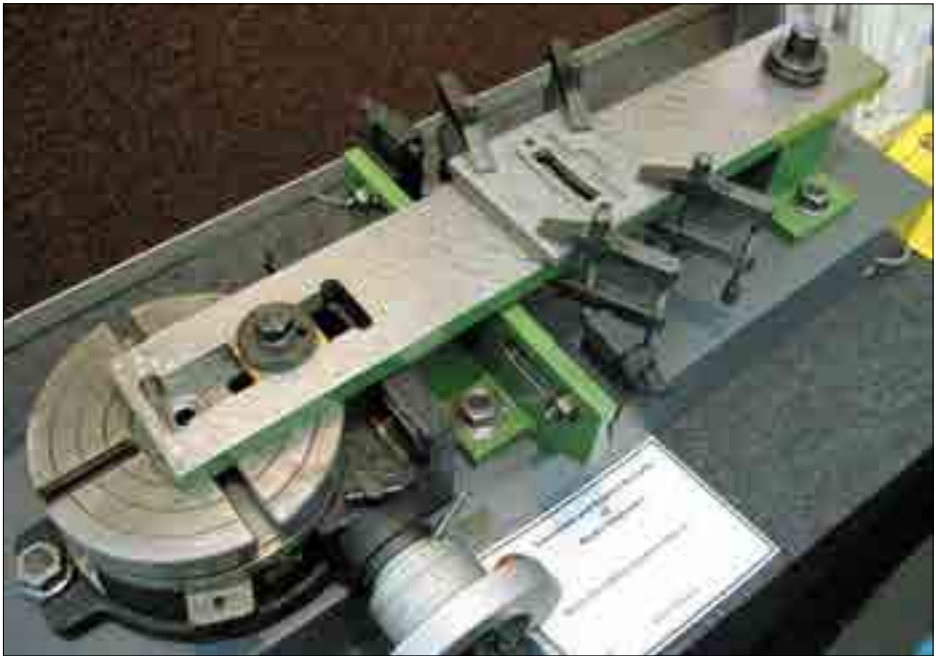
ABOVE: Displayed on the Ickenham & District SME stand at Alexandra Palace, the picture of the Large Radius Milling Attachment, by Peter Pardington, is almost self-explanatory. The 8" radius of the expansion link would require a far larger rotary table than was available. This ingenious device permits far better control, minimising backlash from the worm wheel.
