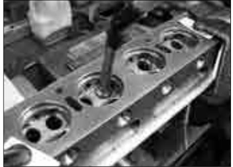
*Finishing the valve seats prior to dry assembly*
