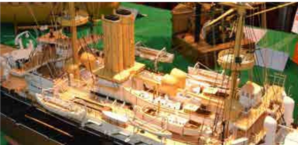
*The ship's boats always carried a sense of pride. Look at the Admiral's pinnace, the Captain's pinnace, all powered by steam. The derricks for hoisting in and out are exact in detail. The ship's boom (for the boats) is visible just above the waterline.*
