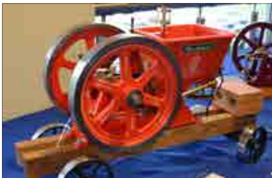
5 HP New Holland "Hit and Miss" engine made by Alan Thatcher from scrap metal with the exception of the flywheels.
