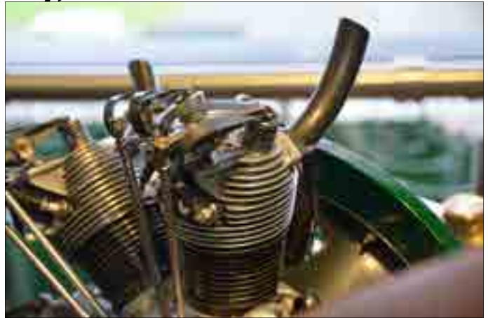
Close up showing detail of a working 1/3rd replica 7 cylinder Radial Armstrong-Siddeley Lynx IV aero engine. by Stephen Wessel.
